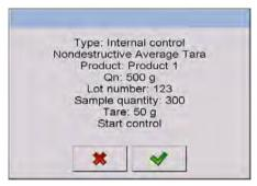
Accept the message box by pressing key which causes moving to the control process. During control process the software carries out real-time monitoring of the measurement results and displays them it the corresponding fields of the display for informing the operator on control result:
