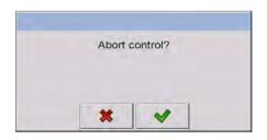
Pressing key means getting back to the control in progress. Pressing key means abort of the control. Abort of control results in getting back to **PGC** mode setting window.
