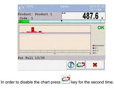
After completing the control the scale generates a process summary, and the accomplished control is automatically saved in the scale database:
